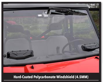
Designed to provide long lasting, scratch resistant, visibility. It includes two independently adjustable vents for driver and passenger comfort. An optional electrical wiper is available.
