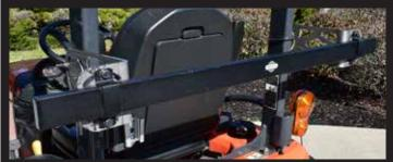
The mounting brackets allow the bar to stay parallel to the ground no matter what angle a given rops structure has in either direction, providing true universality.
