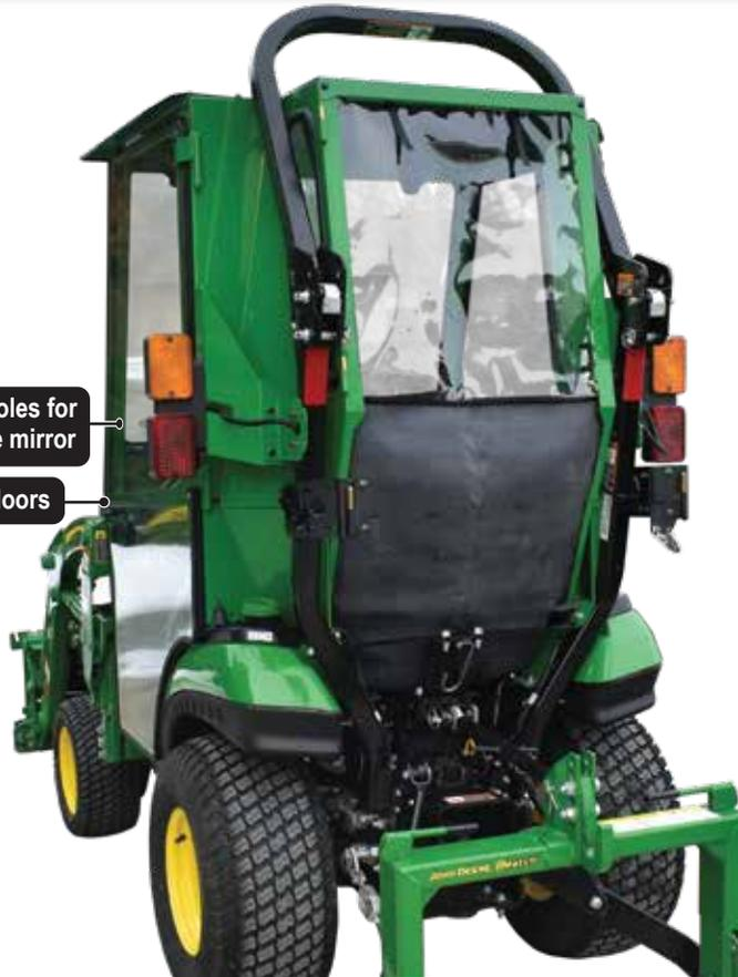
Pre-drilled holes for optional side mirror
