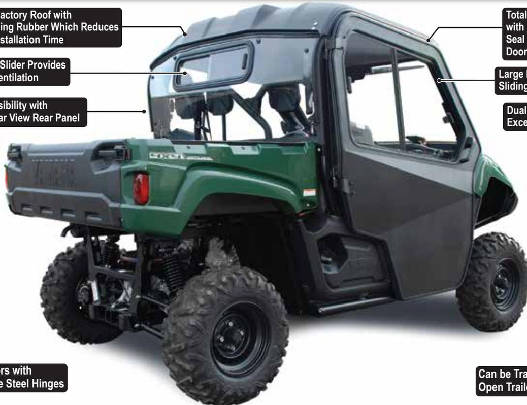
16 Gauge Steel Doors with Heavy Duty 7 Gauge Steel Hinges
