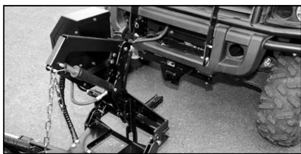
Fig. 2.2—Lift Frame and Receiver Setup
