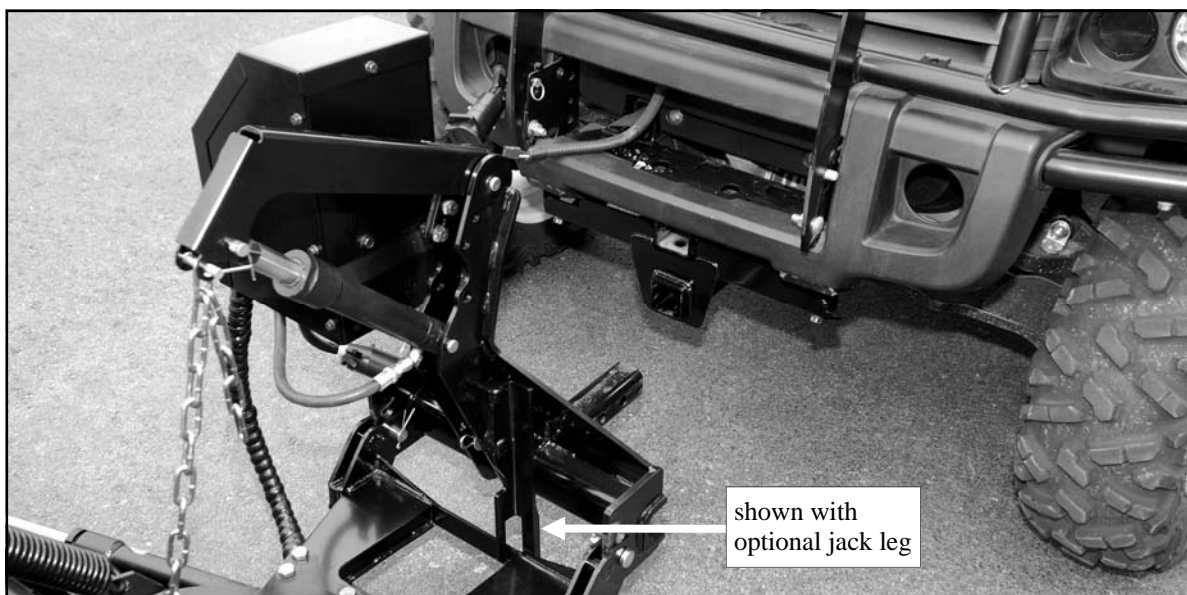
Fig. 1.1—Lift Frame and Receiver Setup
