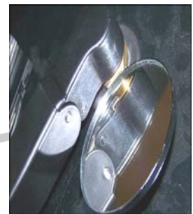
Fig. 3.6.1 shows the wiper arm properly installed (spring clip has sprung down behind/below the raised splines)
