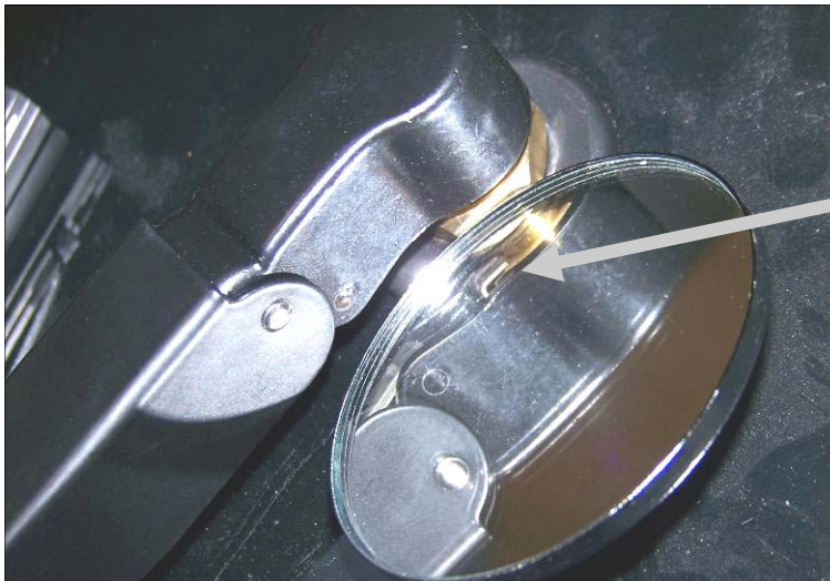
Fig. 3.6.1 shows the wiper arm properly installed (spring clip has sprung down behind/below the raised splines)
