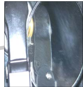
Fig. 3.6 shows the wiper arm not properly installed (spring clip has not sprung down behind/below the raised splines)
